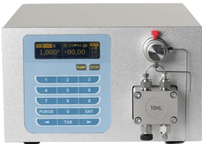
High pressure infusion pump is the core component of accurate liquid material transportation. Widely used in pharmaceutical, fine chemical, green chemistry, catalytic reaction, high molecular chemistry, petrochemical, food, energy, environment, materials and other fields.
